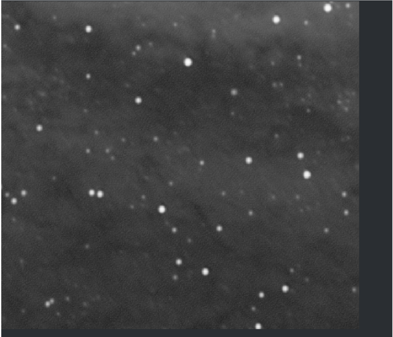
Fig. 30: Close-up showing the effect of trying to apply too much regularization ( \alpha = 30 ) using the multiplicative version of Richardson-Lucy. For strong regularization and / or better control over each iteration, the gradient descent formulation is recommended.
