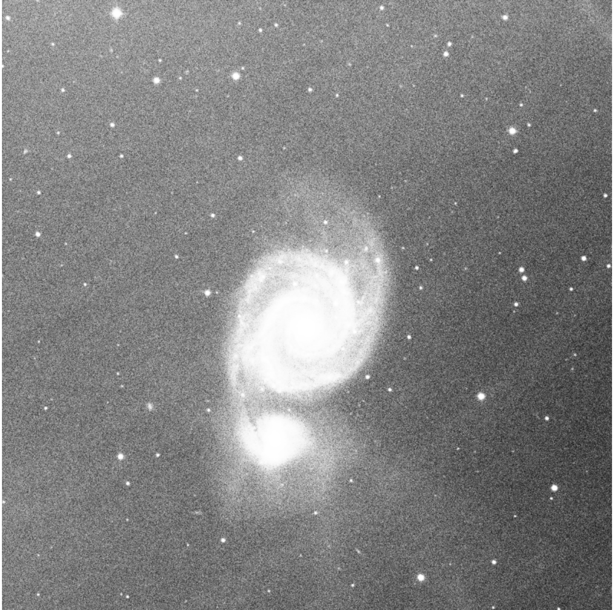
Fig. 12: Thanks to dark optimization, calibration is correct. The only residue visible is CCD fringing in the near IR range, which cannot be removed by calibration. The image is displayed in histogram equalization mode, to highlight any defects.
