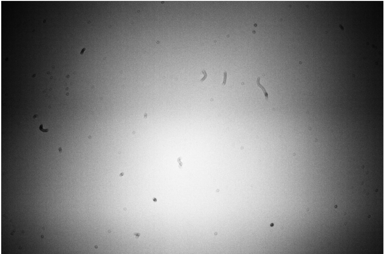
Fig. 13: Example of a flat frame that was shot with a Canon EOS 1100D. The dust present on the optical path, and especially on the sensor, are clearly visible. The vignetting (darkening of the corners of the image) is also very visible. The defects are exaggerated by the viewing mode. Also, the grey_flat command was used on this image to get rid of the Bayer pattern.
